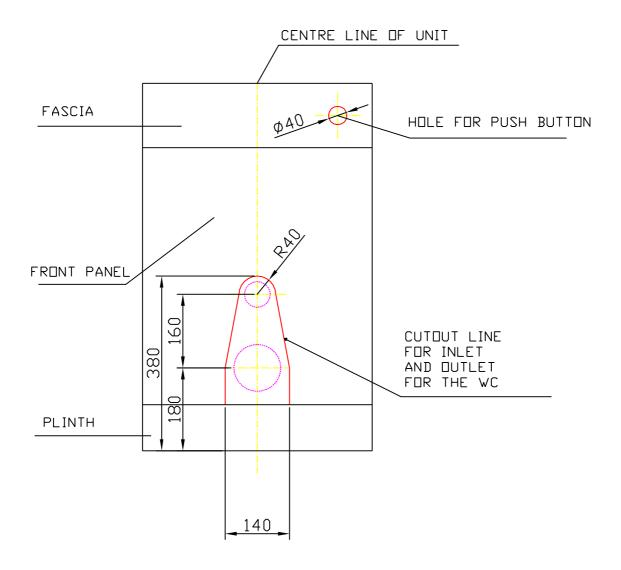
MARK OUT THE OPENING ON THE FRONT PANEL FOR THE INLET AND OUTLETS OF THE WC PAN, BY FOLLOWING THE ABOVE DIMENSIONS, CHECK THE SIZE AGAINST THE PAN BEFORE CUTTING OUT. DO NOT CUT THE BOTTOM PLINTH
