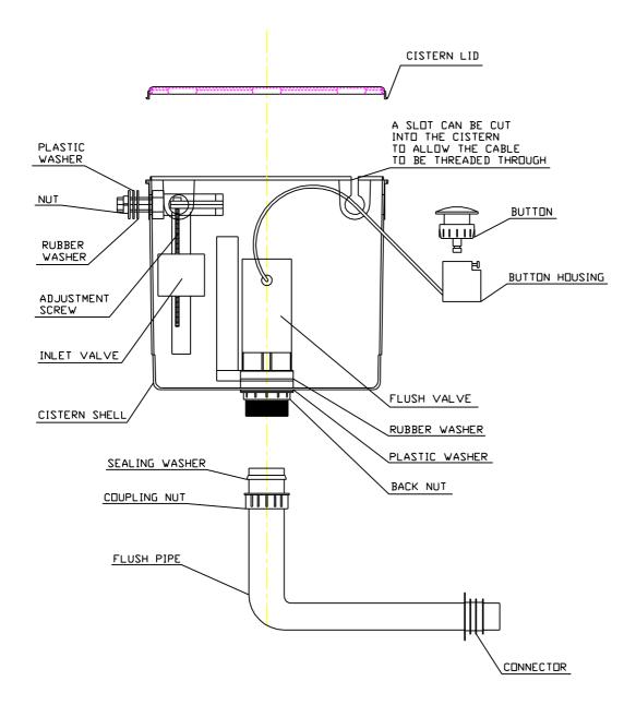
ASSEMBLE THE CISTERN AS ABOVE AND MARK POSITION OF WHERE THE CISTERN IS TO BE FITTED. USE THE BRACKET AND FIXING HOLES TO FIX THE CISTERN INTO W.C UNIT OR WALL CAVITY.
