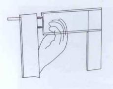
Connect up & down rails with side aluminum and tighten screws, make up aluminum frame
