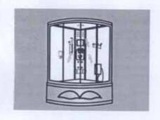
Connect the glass door with the glass backboard, then fx the top
