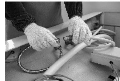
3. Distinguish water inlet pipe
